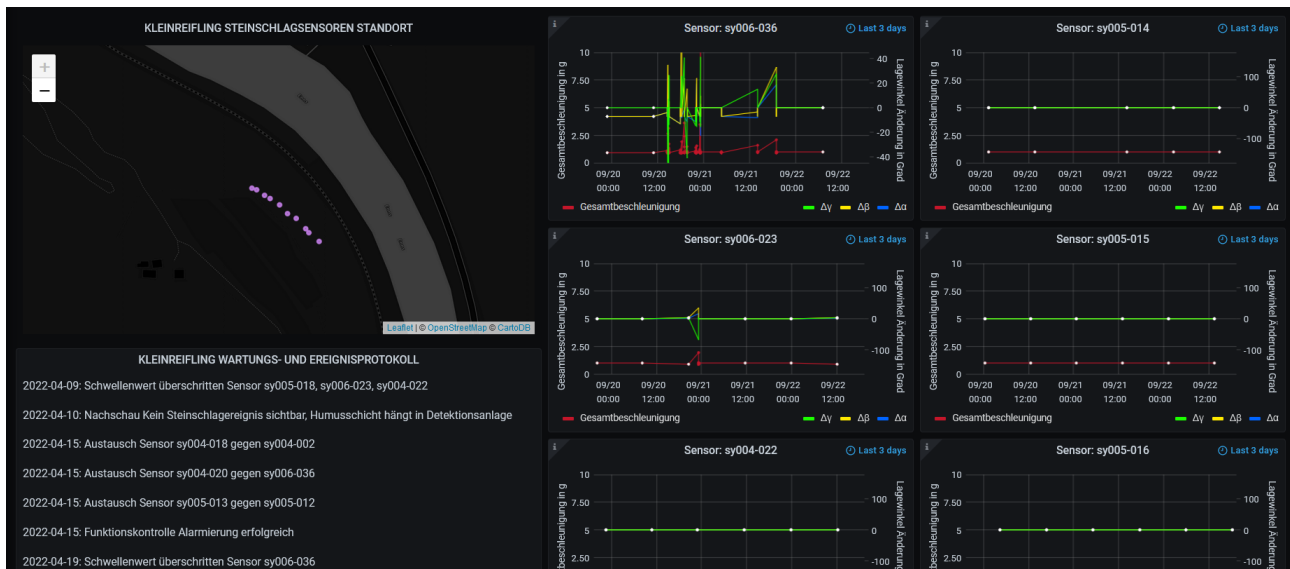
Figure 3 View of a Grafana dashboard for a rockfall project showing an aerial map of location of installed sensors (left panel) and magnitude of measured acceleration along with rotation around cartesian axes respect to the latest wakeup outside the visualized time interval for each sensor (right graphs). The white points are the wakeup measurements.
